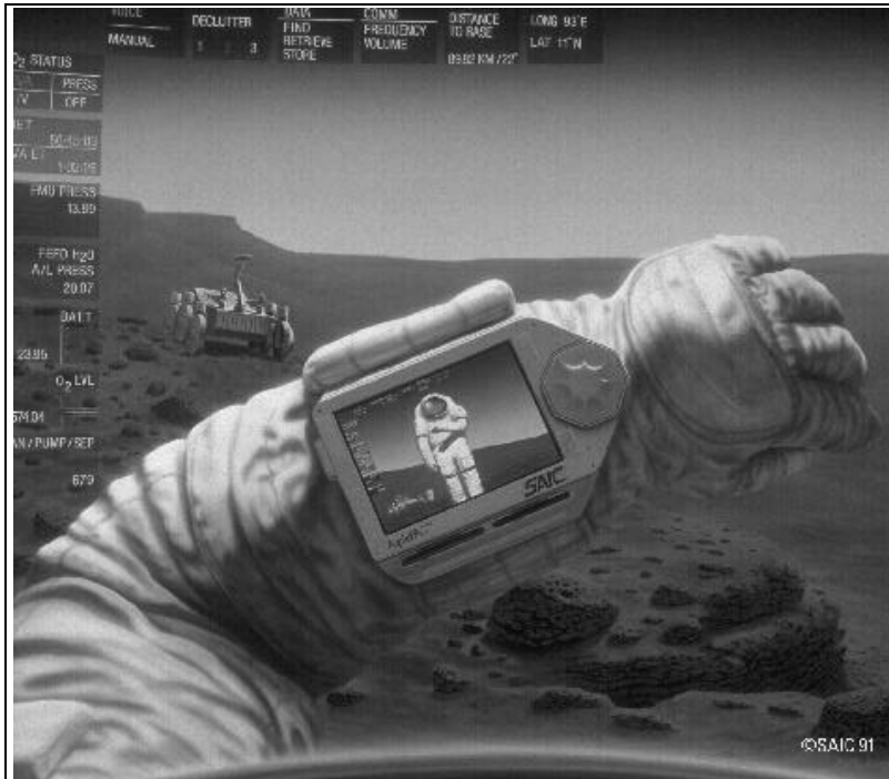
Figure 2.9-1 An EVA crew member peers at his own image as transmitted by a teleoperated rover in a wrist-mounted display and control system. The crew will be able to use control systems similar to this as a means of operating robots that accompany the crew into the field. (© SAIC)
