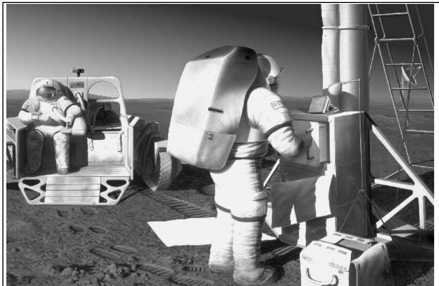
Figure 2.19-1 An EVA crew member changes a faulty line replaceable unit on one element of the surface infrastructure. EVA-accessible enclosures and compatible disconnects will be necessary to allow for effective use of crew time during maintenance and repair activities. (© Lockheed Martin)
