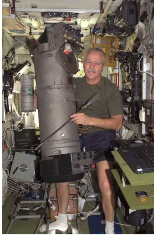
Figure 9: Astronaut John Phillips on ISS Expedition 11 Performing Repairs on the Russian ELEKTRON O 2 Generation System
